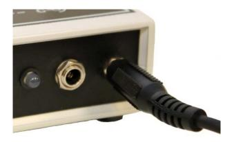
Connect one end of the 3.5mm cable into the jack on the Proximity Control Module labeled OUTPUT JACK and the other end into the device that you want to control.
