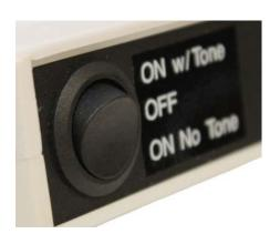
Set the power switch to either ON w/Tone or ON No Tone. With the power switch set to ON w/ Tone you will hear a beep from the Power Control Module each time the sensor is activated. With the power switch set to ON No Tone you will not hear a beep from the Power Control Module.
