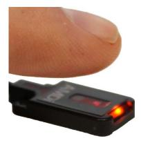
Test the sensor to make sure it is working before you set it up for the end-user. When your finger comes in range of the target area of the sensor LED on the top of the sensor will light Yellow.
