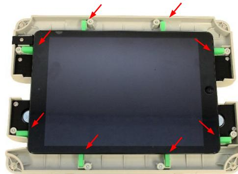
Make sure that the reset button of the iPad® lines up with the reset button of the iAdapter™ as shown in the picture to the right.
