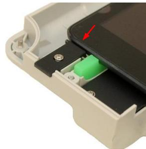
Place the top housing of the iAdapter™ over the iPad®. Align the top housing of the iAdapter™ with the bottom housing of the iAdapter™. Carefully hold both the top and the bottom housing of the iAdapter™ together and then turn it over onto a flat surface. Tighten the 12 (twelve) screws that will hold the iAdapter™ together.
